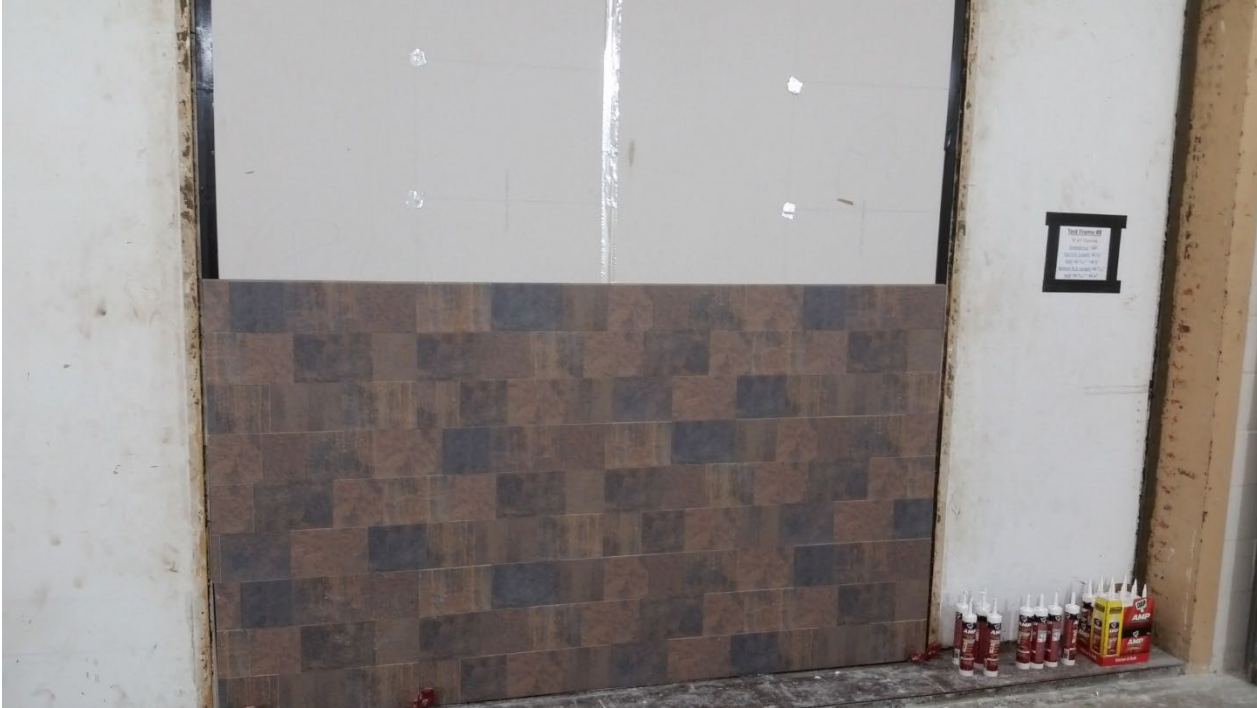
Figure 9 – Decorative wall panels partially installed on source room side
