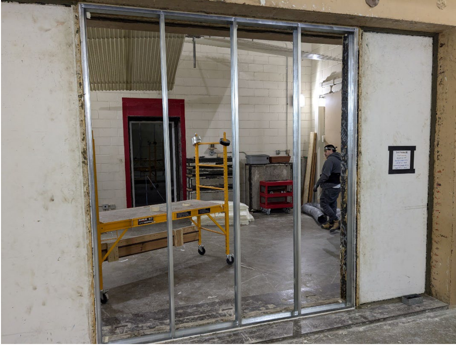
Figure 3 – Tracks and studs installed in test aperture
