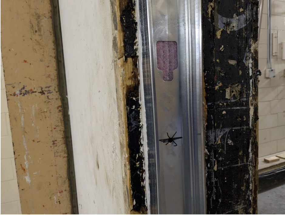
Figure 5 – Detail of side stud fastened to test frame
