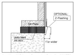
Joto-Vent AND Insect Prevention Strip should NOT be exposed and covered by proper flashing in order to prevent water leaks into the crawl spaces.
