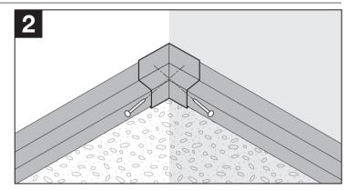
Joint-cover: install by using stainless-steel nails as shown in the illustrations.
