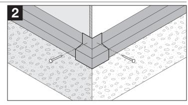
**Inside-corner:** install by using stainless-steel nails as shown in the illustrations.
