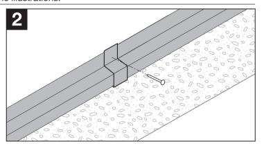
**Endcap:** install by using stainless-steel nails as shown in the illustrations.
