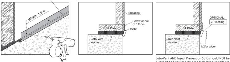
Joto-Vent AND Insect Prevention Strip should NOT be exposed and covered by proper flashing in order to prevent water leaks into the crawl spaces.
